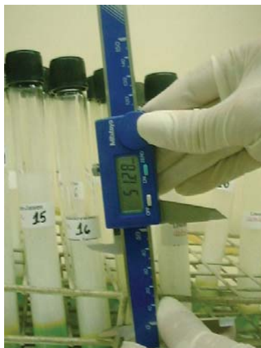
Figure 6 – Semi-quantitative catalase test. The column of foam is above 45 mm yielding a positive semi-quantitative catalase test.
