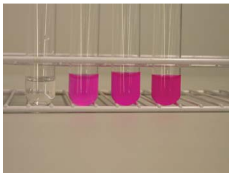
Figure 7 - Acid phosphatase test. The tube on the left shows a negative result; the other three tubes show positive results.
